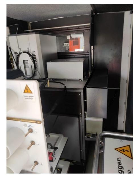
4. Passive Voltage Decoupling , method: voltage decay , Typically for long PILC cables, TDR used in a passive mode as a transient recorder of the voltage on the HV return after the flashover at the fault location, which was initiated by the HV DC source.
