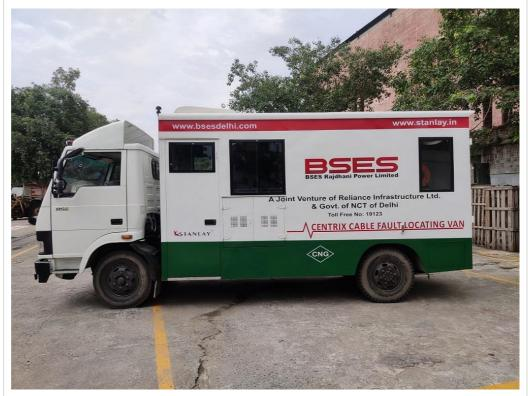
Equipped with the latest generation of cable diagnostics in conjunction with powerful VLF testing technology, Centrix 2.0 makes it possible to perform standard-compliant cable testing with accompanying partial discharge diagnosis
